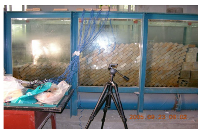
图3 水下边坡模型试验过程 Fig.3 Process of model test of underwater rock slope
